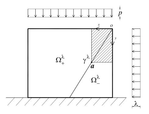
The singularity curve  $\gamma^{\lambda}$  can be obtained by imposing the equilibrium of the shaded rectangular region with the respect to the rotation about its left lower corner. We obtain
